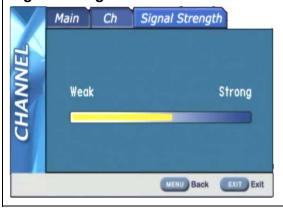
This page also displays from the Signal remote command. The graphic shows the current signal strength, and changes in real time. This allows you to monitor the strength of a channel as you adjust the antenna for best reception.
